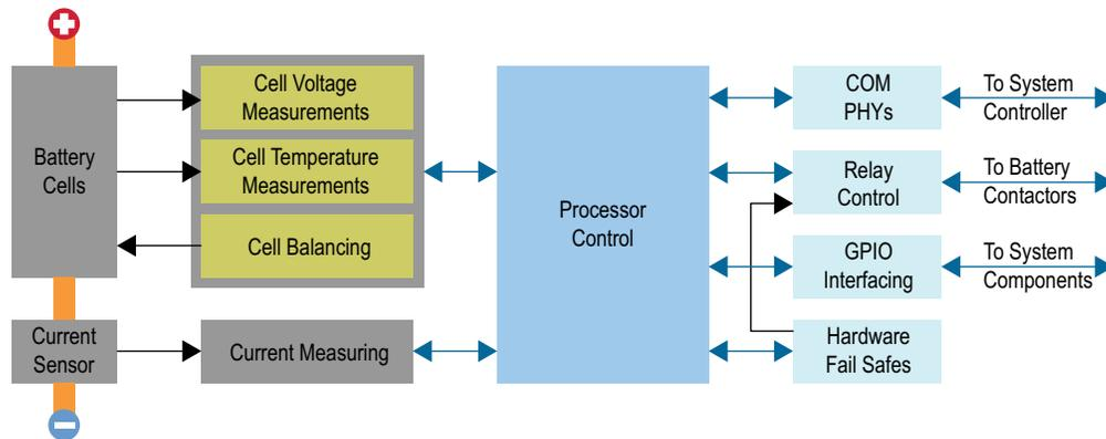
On the left side of Figure 3 are the battery cells, current sensor and data acquisition portion of the BMS. The cell voltage and temperature measurements, and cell balancing are shown with a dotted box around these functions because there are various multicell battery monitor ICs that perform these functions with the addition of some external components. Similarly, there are ICs available that perform current measurement and coulomb counting.
