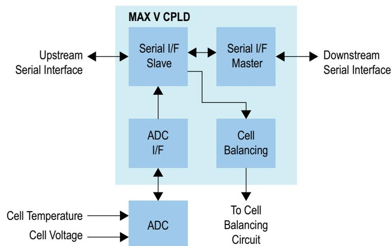
The serial I/F slave and serial I/F master blocks interface with the daisy-chained serial network. The analog-to-digital (ADC) I/F block controls an external ADC to measure cell voltage and temperature. The cell balancing block receives instructions from the master board processor to control external cell balancing circuitry.
