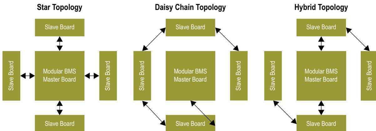
The serial networks can be a star topology or a daisy chain topology or a hybrid of both network types, in which the master control board supports a number of serial daisy chain networks. The topology of the serial networks in the BMS depends on the application. Daisy chain networks provide scalability, but also increase the required serial network bandwidth for systems with a high number of slave boards.
