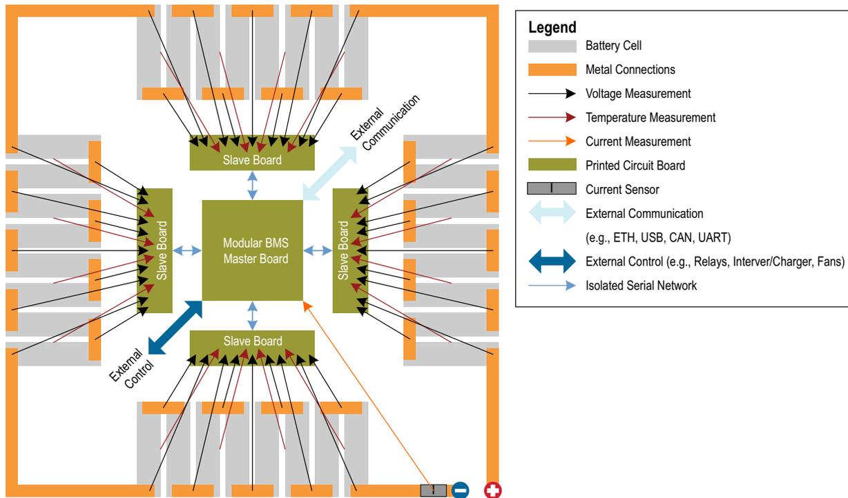
In addition to the master-slave modular BMS architecture, there is also a peer-to-peer modular BMS architecture. In the Peer-to-Peer modular BMS architecture, there is no master board, and each peer board monitors and controls its own set of battery cells and communicates with other peer boards in the system. This architecture divides the software tasks amongst the peer boards, but does require additional software for communication and coordination among peers.
